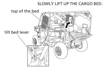
To lower the cargo bed, make sure that the area under the front of the cargo bed is clear, then manually push down on the top of the bed.
