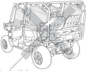
check for exhaust leakage
