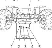
The spring pre-load adjuster has 5 positions for different load or driving conditions. Before adjusting the spring pre-load, jack up your Honda SXS (page 144) to avoid damaging the adjusters.
