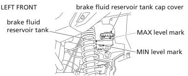
It should be between the MIN and MAX level marks. If the level is at or below the MIN level mark, check the brake pads for wear (page 199).
