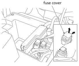
brake traction control system (BTCS) fuse
