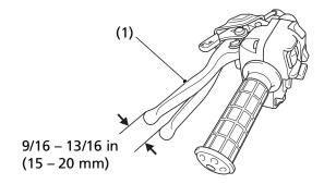
(1) rear brake lever/parking brake lever
