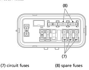
6. To check or replace a circuit fuse (7), pull the old fuse out of its retaining clips.
