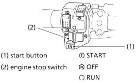
The start button (1) is used for starting the engine. Pushing the button in starts the engine. See *Starting Procedure*, page 72.
