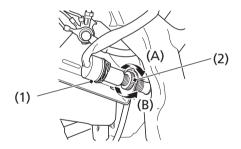
(1) rear brake light switch (2) adjusting nut
