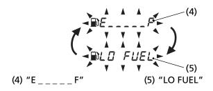
When the fuel gauge show " $E_{---}F$ " (4) and "LO FUEL" (5) blink 3 times alternately and fuel mark blinks, you should refuel as soon as possible.
