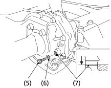
(5) oil level check bolt(7) oil level check hole(6) sealing washer
