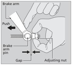
After adjustment, confirm the freeplay of the brake pedal.
