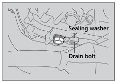
**6.** Install a new sealing washer onto the drain bolt. Tighten the drain bolt.
