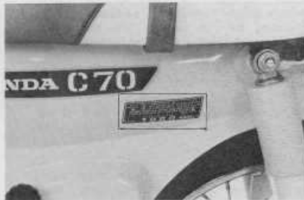
The Vehicle Identification Number is on the Safety Certification Label on the frame's left side.
