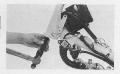
Apply a coat of bearing grease to the upper ball race and install 21 steel balls.
