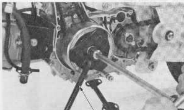
FLYWHEEL HOLDER 07922-1790000 U.S.A. ONLY - USE COMMERCIALY AVAILABLE BAND STRAP WRENCH
