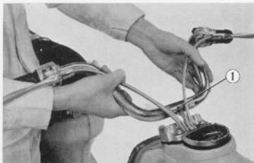
Fig. 4.14 Removing steering handle (CD 90 & CT 90) ① Handle bar
