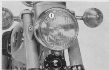
Fig. 4.25 Removing headlight ① 8×22 hex bolt
