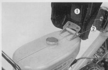
Fig. 4.53 Removing seat hinge pin ① Seat ② Seat hinge pin
