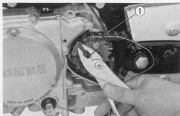
Fig. 4.94 Disconnecting drive chain ① Drive chain
