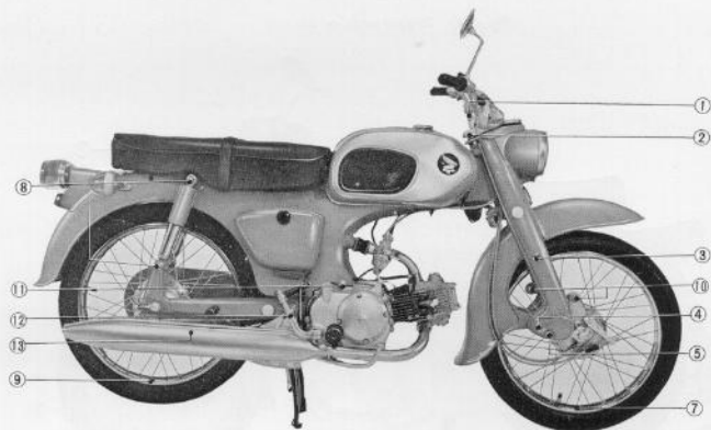
Fig. 5.42 Torquing points on right side
