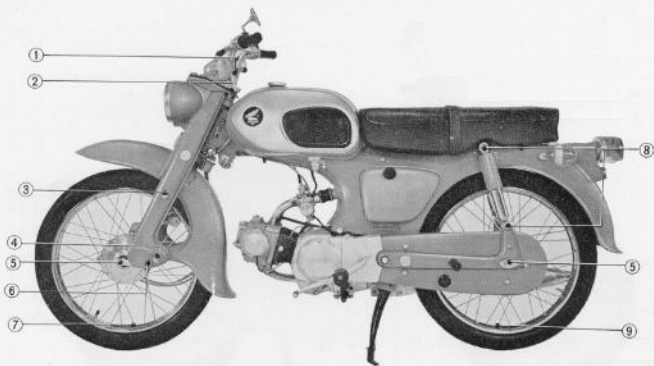
Fig. 5.41 Torquing points on left side
