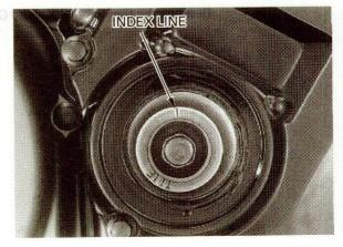
Record the clearance for each valve for reference in shim VALVE CLEARANCE: selection if adjustment is required.
