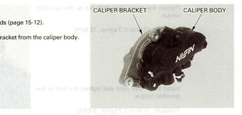
Remove the brake pad spring from the caliper body. Remove the brake pad retainer from the caliper bracket.
