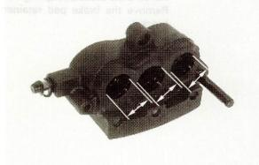
Check the caliper pistons for scratches, scoring or bod regise by a stod of a scratches other damage.
