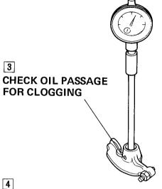
Measure the amount of wear on the rocker arm I.D. with an inner dial gauge. Take measurements at two positions crosswise of each other.
