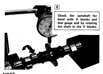
7 | T.I.R. (Total Indicator Reading) should be divided by 2 to determine the actual bend taking place in the shaft.
