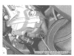
**IDLE SPEED:**  $1,300 \pm 100 \text{ min}^{-1} \text{ (rpm)}$
