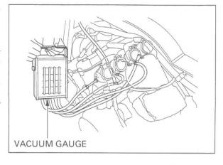
Synchronize to specification by turning the adjusting screw with the philips screwdriver.
