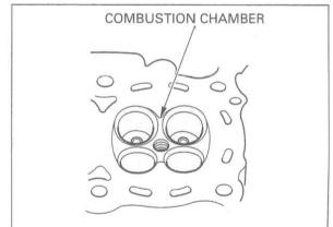
Check the cylinder head for warpage with a straight edge and feeler gauge.
