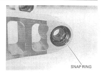
Press the right pivot bearings (radial ball bearings) out from the swingarm pivot using the special tool.
