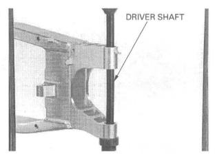
Press the left pivot bearing (needle bearing) out of the swingarm pivot using the special tools.
