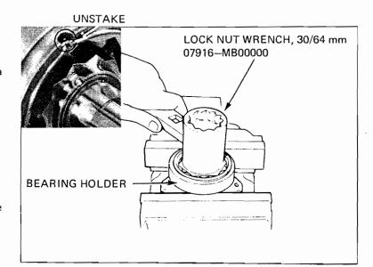
Place the bearing holder in a press and remove the bearing.
