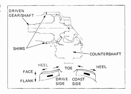
If the pattern is not correct, remove and replace the driven gear adjustment shim. Replace the shim with a thinner one if the contact pattern is too high.
