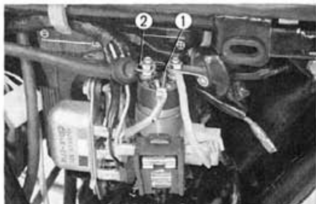
Fig. 9-3 ① Magnetic switch ② Starting motor cable
