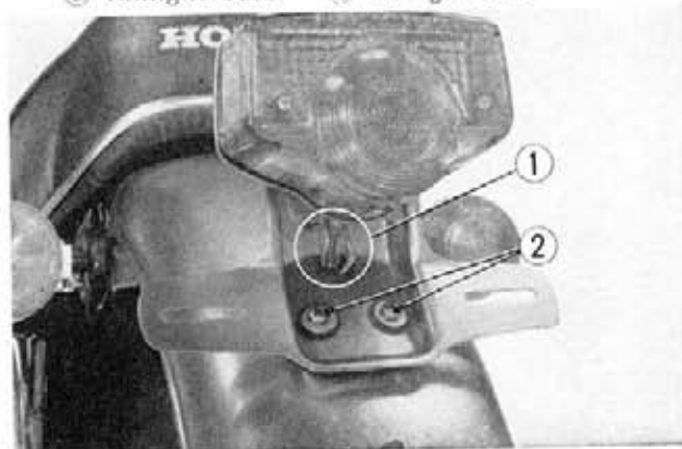
Fig. 16-7 ① Lead connectors ② Taillight bracket screws
