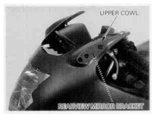
Disconnect the headlight sockets and position light connector, then remove the upper cowl.
