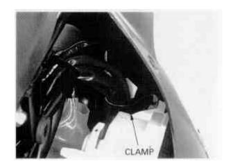
Remove the trim clips between the upper cowl and ram duct.
