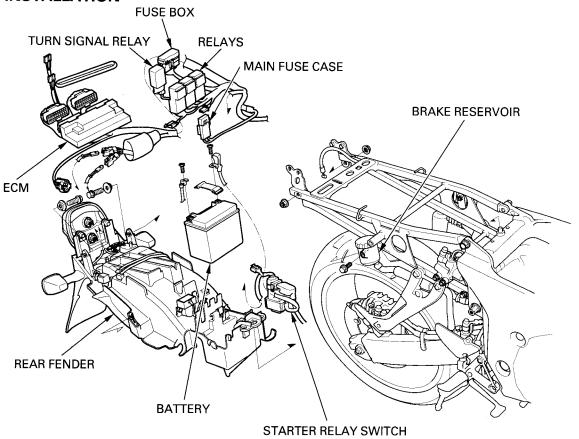
Install the rear fender into the seat rail, while aligning the front groove of the rear fender with the cross bar.
