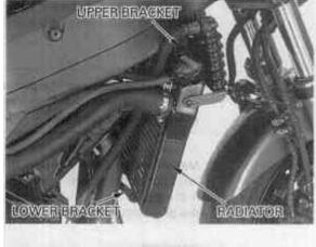
Install and tighten the radiator upper mounting bolt. Connect the fan motor sub-harness 2P (Natural) connector.
