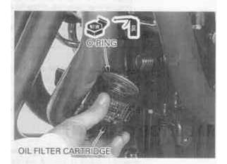
Install the new oil filter and tighten it to the specified torque.
