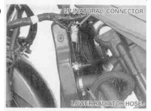
Remove the radiator mounting bolt.
