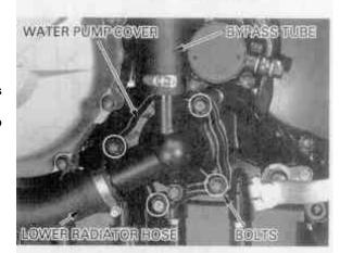
Remove the O-ring from the water pump body. Remove the water pump body from the crankcase.
