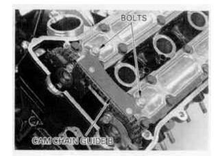
Loosen and remove the camshaft holder bolts, then remove the camshaft holders and camshafts.
