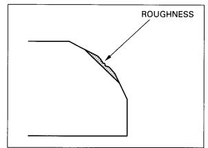
Use a 32-degree cutter to remove the top 1/4 of the existing valve seat material.
