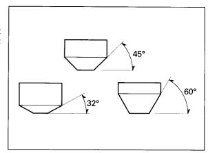
Reface the seat with a 45-degree cutter whenever a valve guide is replaced.
