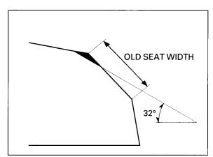
Use a 60-degree cutter to remove the bottom 1/4 of the old seat.
