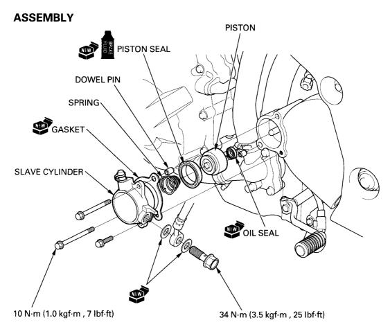
Install the new piston seal with its groove side facing to the slave cylinder.
