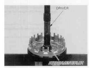
Press a new needle bearing into the clutch outer so that the casing of the needle bearing is flush with the clutch outer surface as shown.
