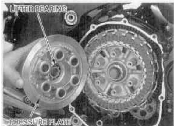
Install the clutch springs and spring bolts.
