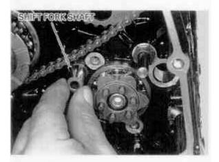
Install the bearing set plates with their "OUT" marks facing out.
