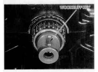
Install the flywheel aligning the key way in the flywheel with the woodruff key on the crankshaft.
