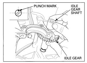
Remove the rear balancer shaft holder bolt. Loosen the pinch bolt and remove the holder.
