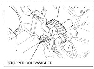
Rotate the balancer idle gear shaft and place the punch mark on the shaft facing down.
