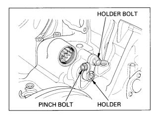
Rotate the rear balancer gear shaft and place the punch mark on the shaft facing down.
