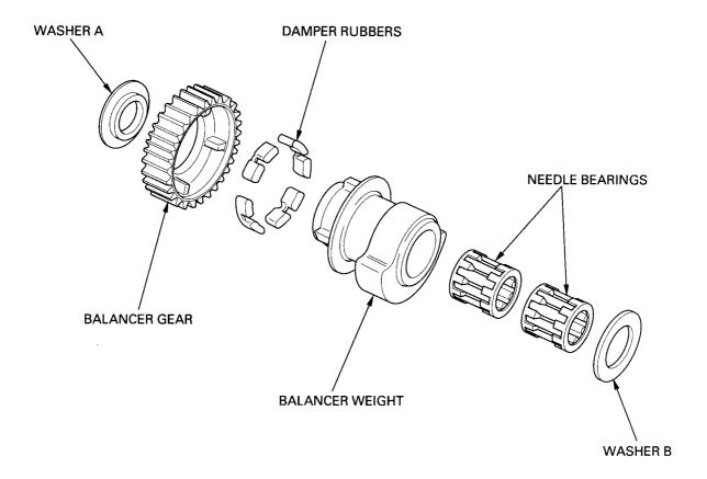
Apply clean engine oil to the damper rubbers. Install the damper rubbers into the groove of the balancer gear.
