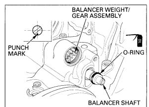
Install the rear balancer shaft holder and tighten the holder bolt to the specified torque.
