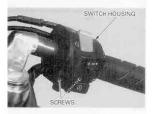
Disconnect the throttle cable ends from the throttle pipe and remove the housing.
