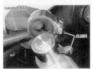
Tighten the left handlebar pinch bolt to the specified torque.
